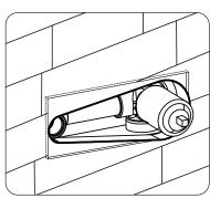
3.Cover the embeded box and fill in the right amount of concrete around the embedded box. When the concreteis dry,cut off the spare cover with a sharp knife along the box border.
