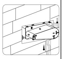
2.Connect the hot flexible hose on the left side of the body while the cold flexible hose on the right. Then turn off the faucet to check if there is leakage from the connector.
