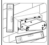
Based on the size of the embedded box, dig a hole at the height of approximately 1100mm from the ground. Install the embedded box with wall-mounted body into the hole. According to the base of using the highest line or lowest line of the box to match the wall, then use horizontal rule to measure whether the box is fixed horizontal or vertical.
