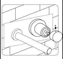
6.Install the handle on the body,tighten the hexagon screw to fix the handle and fill in the stud.
