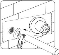
5.Wrap the connector of the spout with sealing tape and install the plate to the spout, then install them on the left hole. Install the plate on the faucet and make to stick to the wall.
